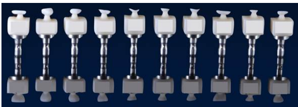
Fig 50. Natural shapes milled in Empress CAD Multi A1
